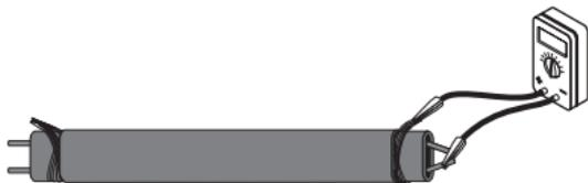
**Figure 11: Capacitance test**
