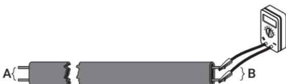
**Figure 13: Measurement of the HWAT cable resistance**
